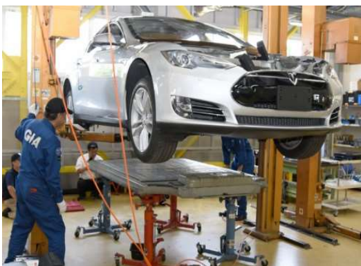
Fig.1. Removing the battery pack from the Model S.
