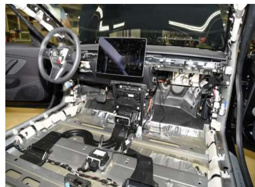
Fig.2. Immediately before the battery pack is removed. It is necessary to remove the seats and floor carpeting, and then unscrew the bolts fixing the battery pack onto the vehicle's chassis.
