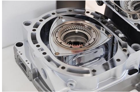
The new rotary engine providing the generative power for the range extender
